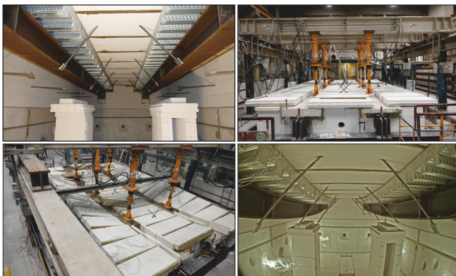
Image 2: Conducting fire tests on steel composite girders at the iBMB (Institute for Building Materials, Solid Construction, and Fire Protection) in Braunschweig
