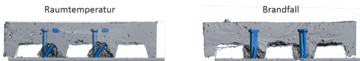
Image 1: 3D scans of pushout specimens before and after testing
