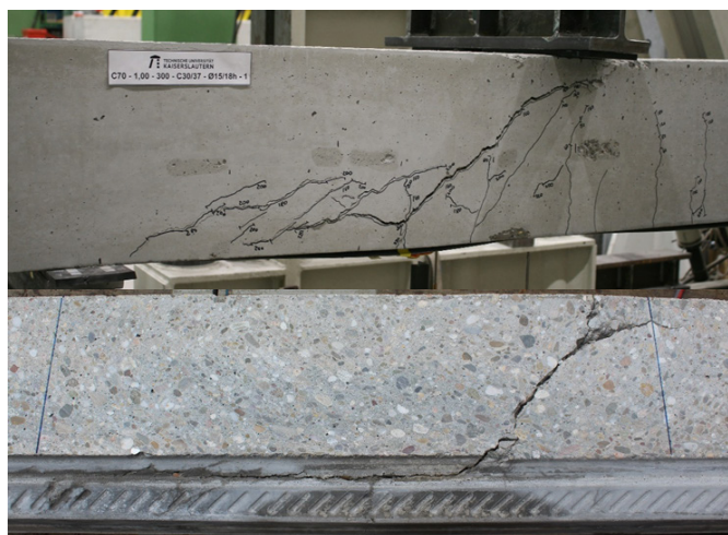
Image 1: Decisive shear crack formation on the component surface and inside a test specimen.
